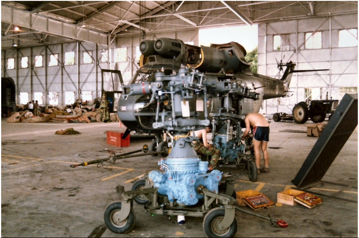
Above: The Unsung Heroes cracking on with a gearbox change at Palenquero Airbase in Columbia. Below: Name the people - from left to right the aircrew were: John Bray-Smith (hand on sponson), Dick Godley (standing on the step), Chris Perkins, John Darby (leaning out of the cabin holding a plaque), Doug Finlay-Maxwell (leaning against the winch), Steve Speight( on Doug F-M's left), Any Swetman (kneeling in front of Dick). Groundcrew nominations, please?
